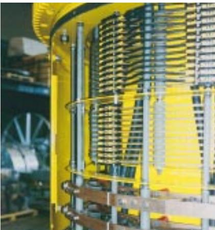
The lower part of the picture shows the power rings with copper bars which connect the brushes. In the upper section 28 control rings are arranged. Both rings and brushes may be prewired to junction boxes (see above illustration). A slewing ring allows an accurate and silent movement. Central passage diameter, enclosure height and other main dimensions may be designed on request to meet customer requirements.
